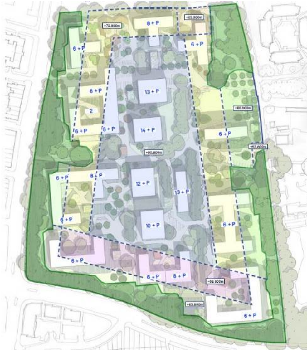
Illustrative Masterplan overlaid on the building height parameters plan (indicative number of storeys of buildings plus roof top plant in blue)
