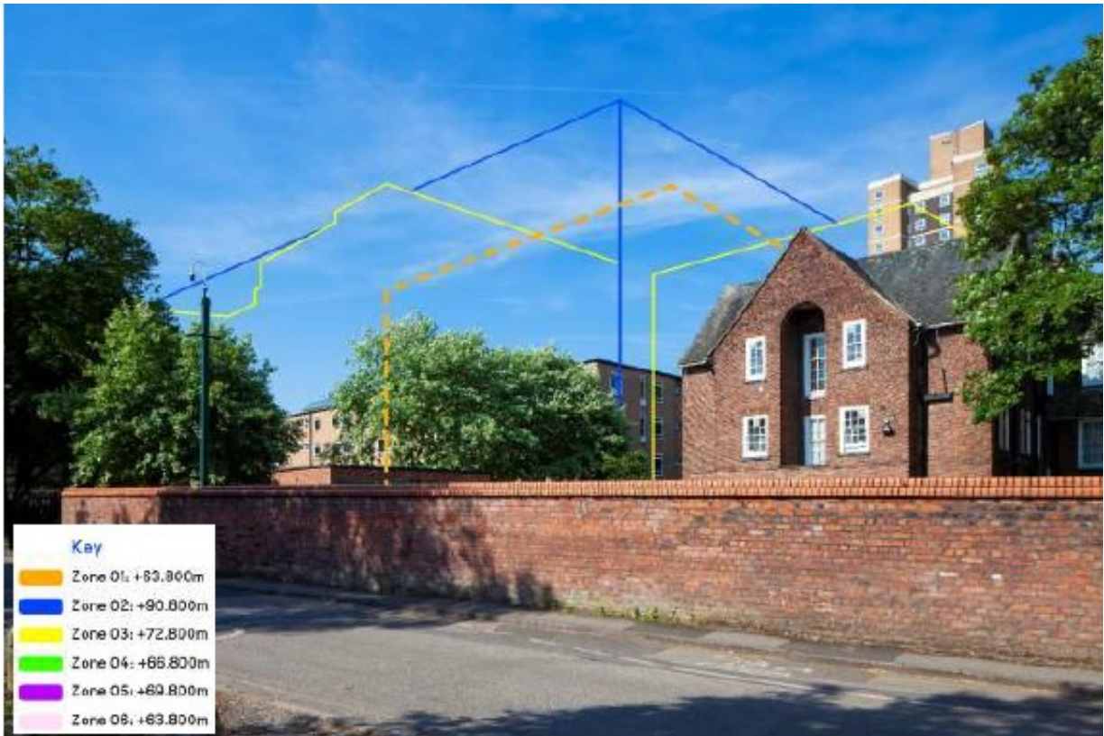
Wireline diagram showing respective heights of proposed buildings set out in the parameters plan view from Whitworht Lane looking south-west – Ashburne Hall to the right with Owens Tower in the background
